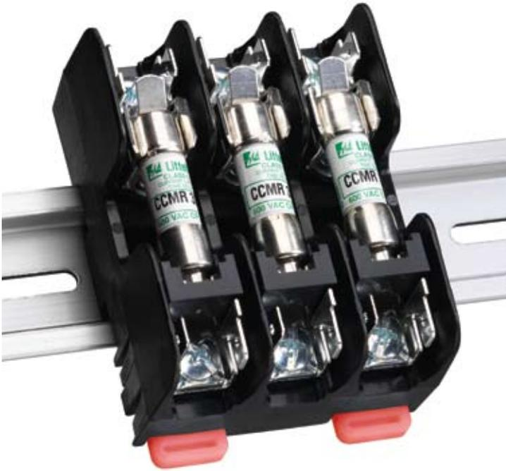
Littelfuse Class CC, G and Midget fuse blocks have integral DIN rail mounting capabilities that allow secure mounting to 35mm “hat” type DIN rails. This new releasable mechanism allows installation and removal of block without removing adjacent components on the DIN rail. Electrical panel builders and machine builders no longer need to use mounting adapters, saving assembly time and related costs.
